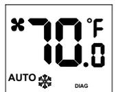
The room temperature is displayed "ROOM". Both setpoint and room temperature displays will indicate the fan speed activity and "DIAG".
