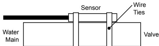
Mount the pipe sensor to the water pipe. The best location is to be as close to the main pipe as possible and attached before the water valve connection.
