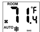
Diagnostic mode can be deactivated by changing the °F/°C slide switch.
